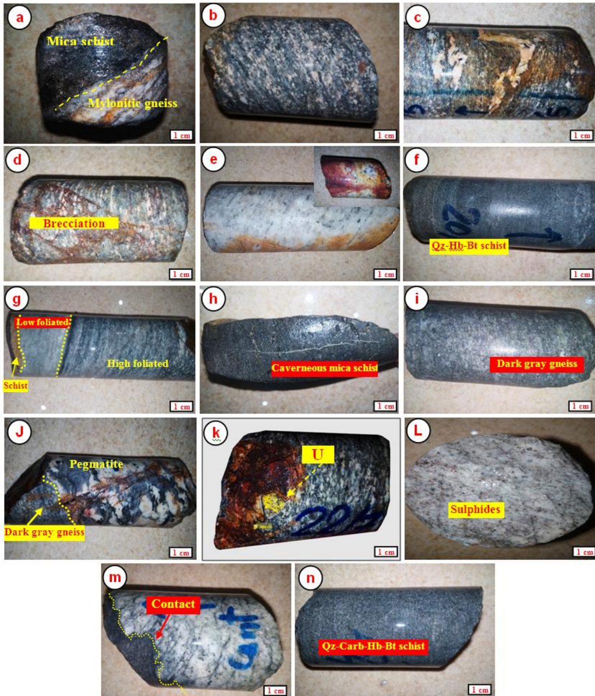
Figure 4: Representative photographs of drill core samples from the studied borehole used in this study: a-Mica schist overlies directly quartz feldspar white mylonite gneiss with sharp contact. b- Well-developed millimeter-spaced gneissic banding in buffish gray mylonite gneiss core samples. c- Pegmatite veinlets dissected along the foliation planes and showing isoclinal microfolds in buffish gray mylonite gneiss. d- Brecciation and ferrugination along the fractures. e- Quartz feldspar white mylonite gneiss core sample. f- Quartz-hornblende-biotite schist core sample. g- High foliated whitish gray mylonite gneiss ended by low foliated zone at the contact with cavernous mica schist. h- Cavernous mica schist core sample. i- Dark gray mylonite gneiss core sample. j- Pegmatite core sample. k- Secondary uranium mineralization associating iron. l- Core sample enriched by disseminated sulphide and black small iron patches. m- Sharp contact between the whitish gray mylonite gneiss and Quartz-carbonate-hornblende-biotite schist. n- Quartz-carbonate-hornblende-biotite schist core sample.
